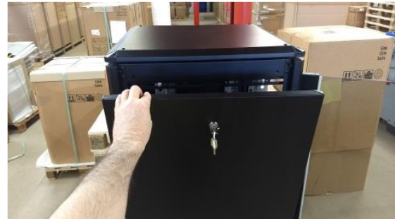
Panel can now be lifted and eased away from the frame.
