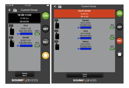
The Recording and Timecode window displays timecode, frame rate, and an absolute record time counter. The window is red when recording and black when stopped. This window is not displayed in RF Only mode. The first transmitter of the group list is used to display the details of the Recording and Timecode window.
